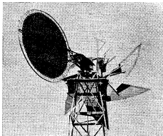
Fig. 12. Sailing rotor of multi-purpose windmill.
